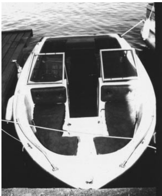
FIG. 2.—Case 2, motor boat which is a 17 ft open bow model without a cabin. The exhaust is located at the stern and vented only at the water level when idling.
